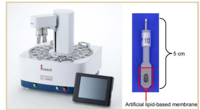
Electronic tongue system (Insent TS-5000Z)
