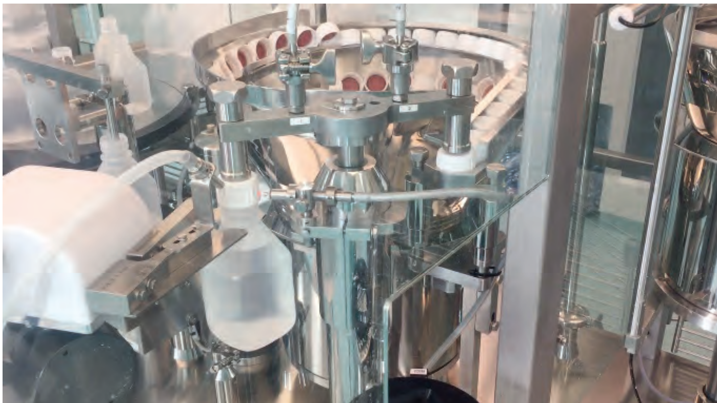
Fig. 3 – The process of closing containers with a screwcap handled by a robotic gripper which could grip vials and containers with different shapes and caps. (Photo Steriline S.r.l.)
