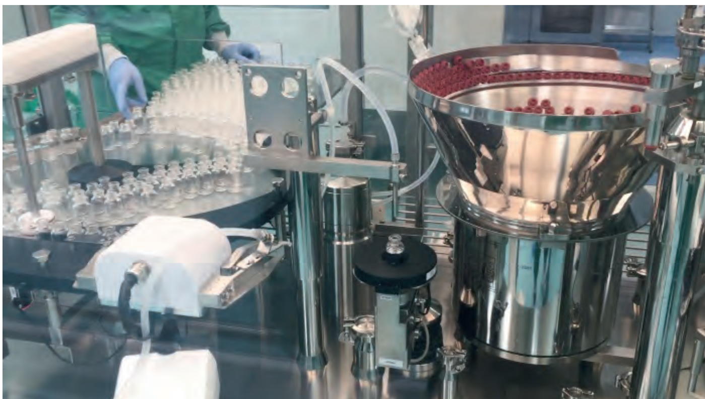
Fig. 2 – The process of filling a little glassware cartridge with the RVFCM. (Photo Steriline S.r.l.)
