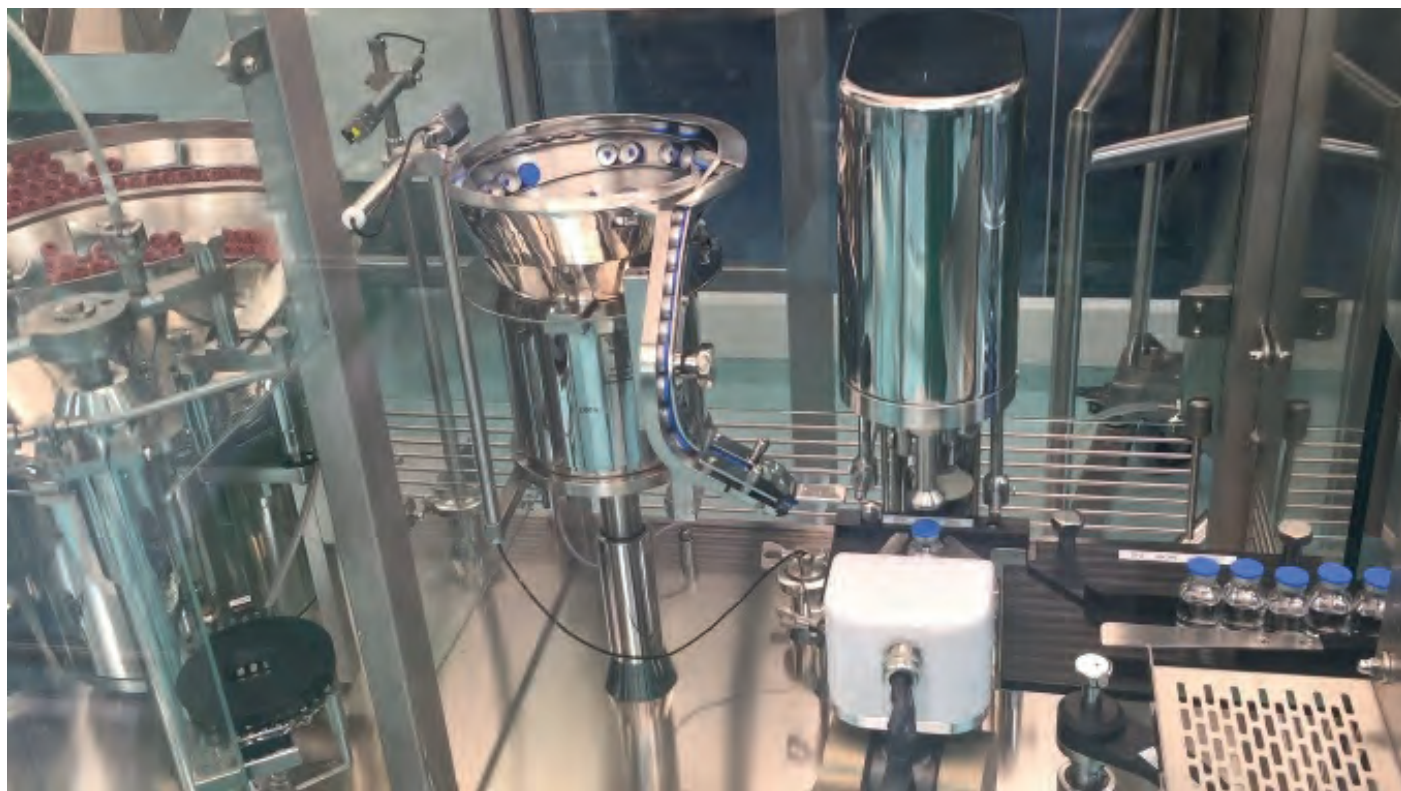
Fig. 4 – The RVFCM stoppering a glassware cartridge. A sensor detects the stopper and cap presence and consequently the machine rejects the un-stoppered vials. (Photo Steriline S.r.l.)
