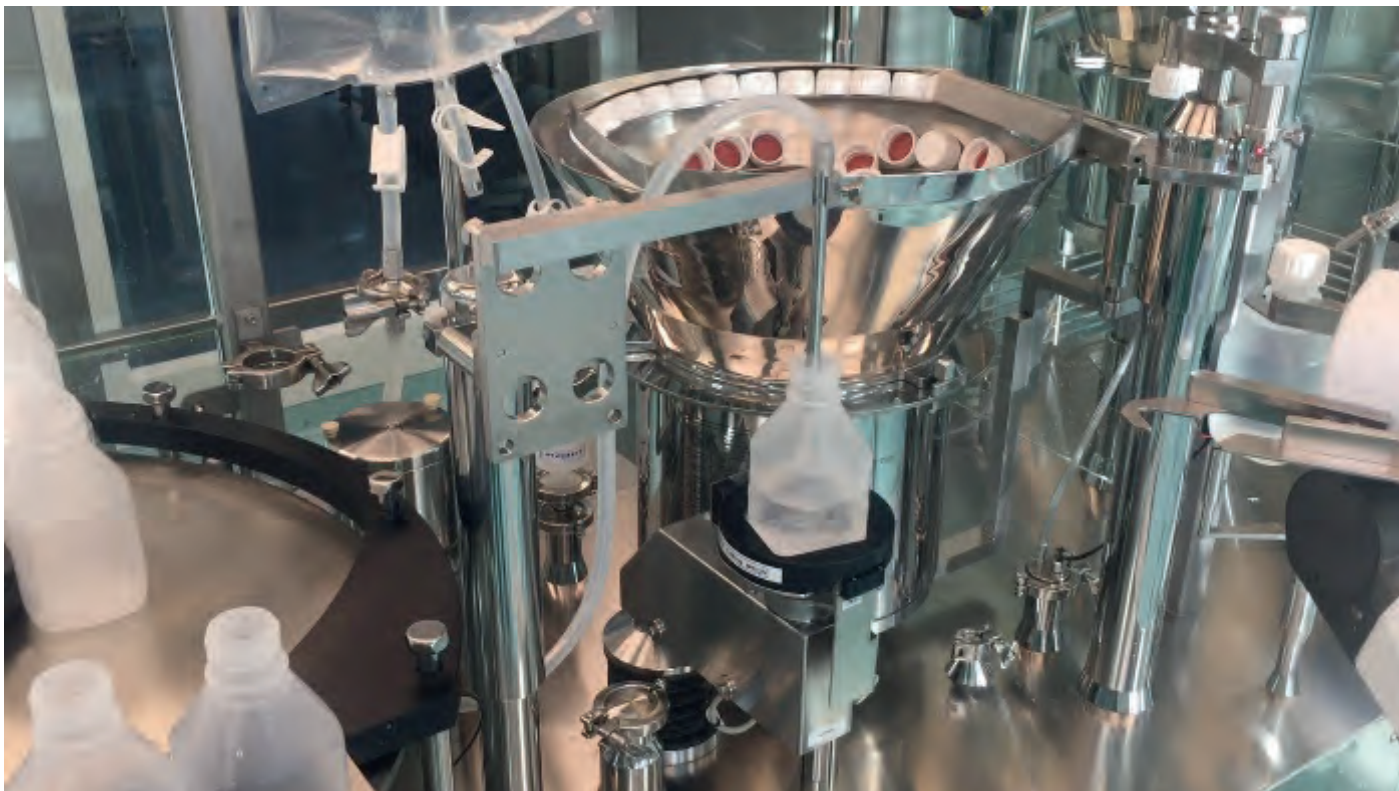
Fig. 1 – The RVFCM filling a 2L plastic container through a net weight filling system, allowing no product waste. (Photo Steriline S.r.l.)
